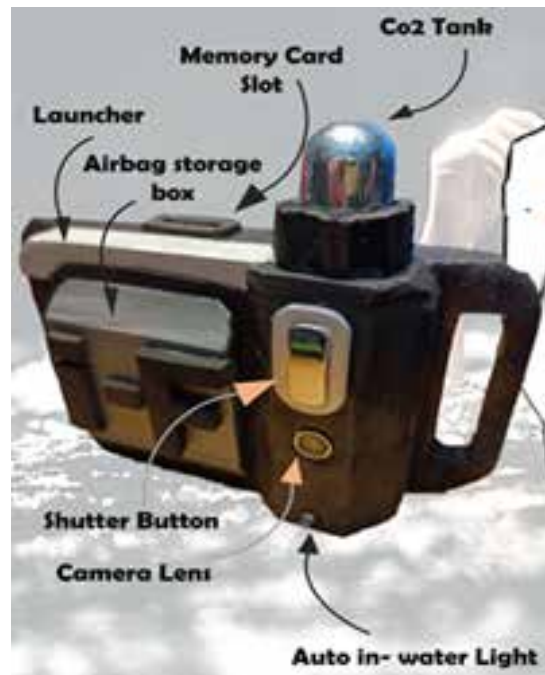
Picture 9: Prototype 3 – I-Float Genesis prototype (Phase 2).
