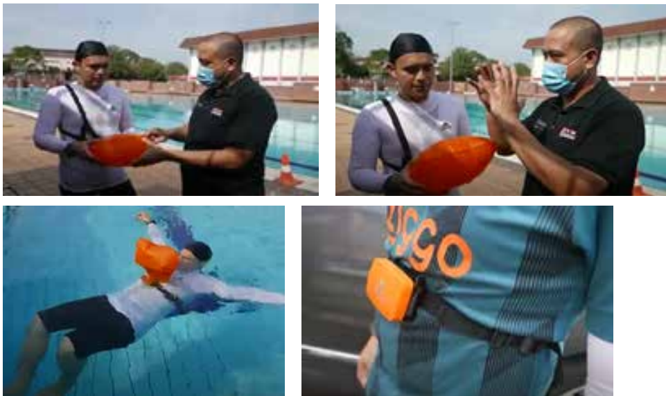
Picture 5: Test. The flotation test carried out on the prototype to identify the body position and deployment of the airbag.
